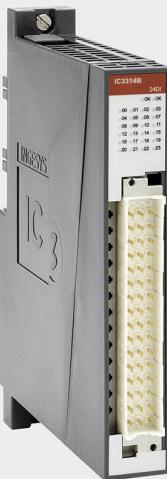
The IC3314 module has 24 digital inputs, 16 x 24Vdc digital inputs with common ground and 8 high-speed digital inputs for up to 4 counters for incremental encoders.
