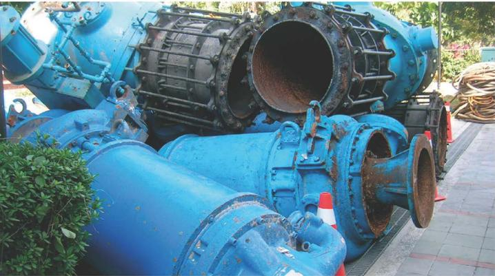
Again, Indar supplied environmentally friendly sets, lighter in weight, compact design ready to be installed (no alignment required), less wear and easier maintenance, less space required, less costly installation (geometry and reduced diameters), IP68 (no risk of electrical short circuit), self-lubricated and cooled, etc.
