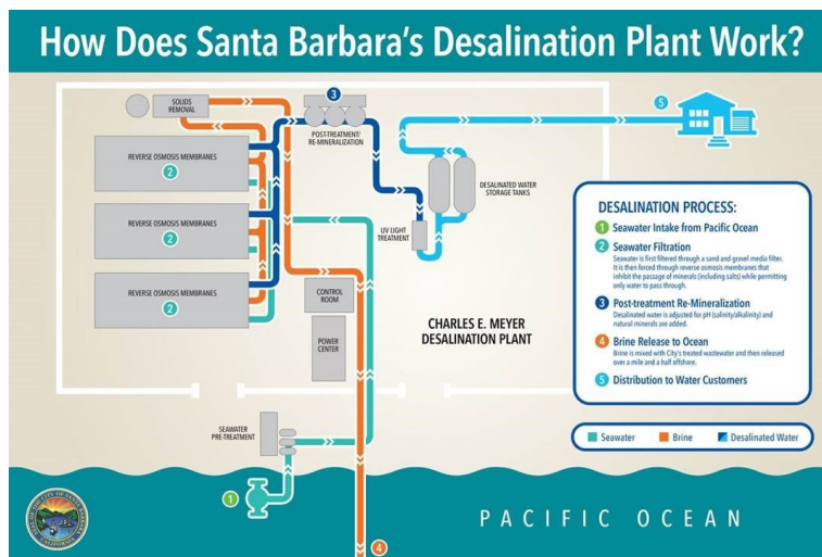
Figure 3: Desalination process in The Charles E. Meyer Desalination Plant Source: City Of Santa Barbara (1) Location of the SeaWater Intake (Open Ocean)
