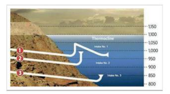
The intake is designed to maintain SNWA's ability to draw water from the Colorado River basin, at lake elevations as low as 300 m above sea level. This will ensure the needed system capacity if lake levels fall below the elevation capacity of the existing PS-1. PS-3 avoids interruptions of continuous water supply to Municipalities and end-users in the event declining lake levels.
