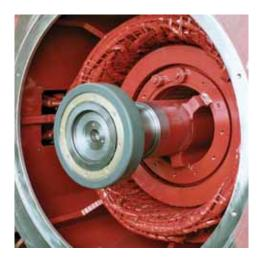
Mounting of insulated bearing to avoid passing current through them
