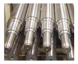
One of the keys for long life motor life consists in that when the motor is operating its vibrations be minimum. This is achieved by manufacturing a robust rotor, and with fine balance.
