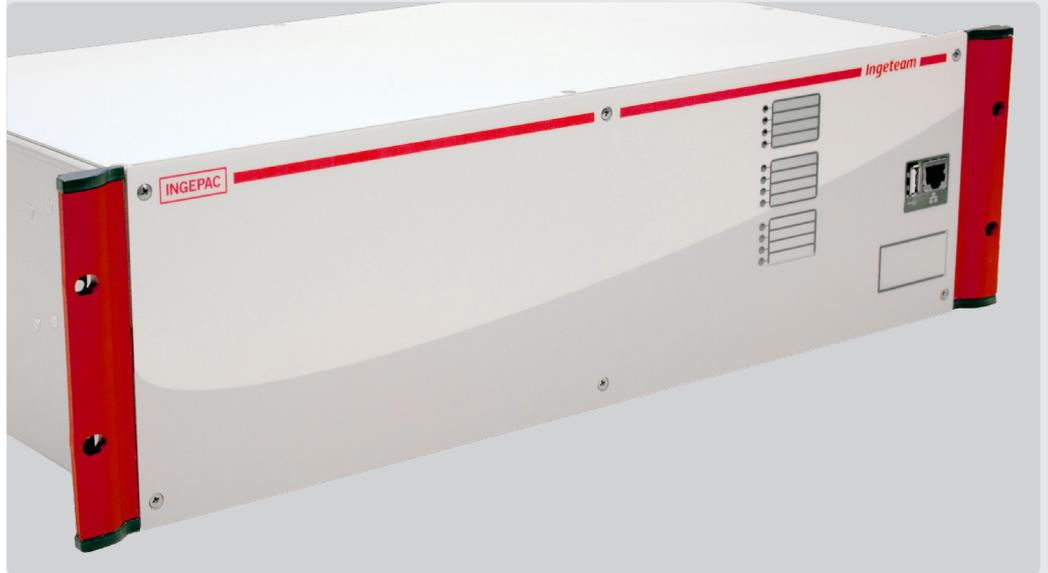
**INGEPAC™ EF PB** is the family of devices that Ingeteam has designed as a SAMU (Stand Alone Merging Unit); the device acquires conventional transformer currents and voltages (CT and VT), and **converts them into digital values**, transmitting them to an Ethernet network, also called a process bus.
