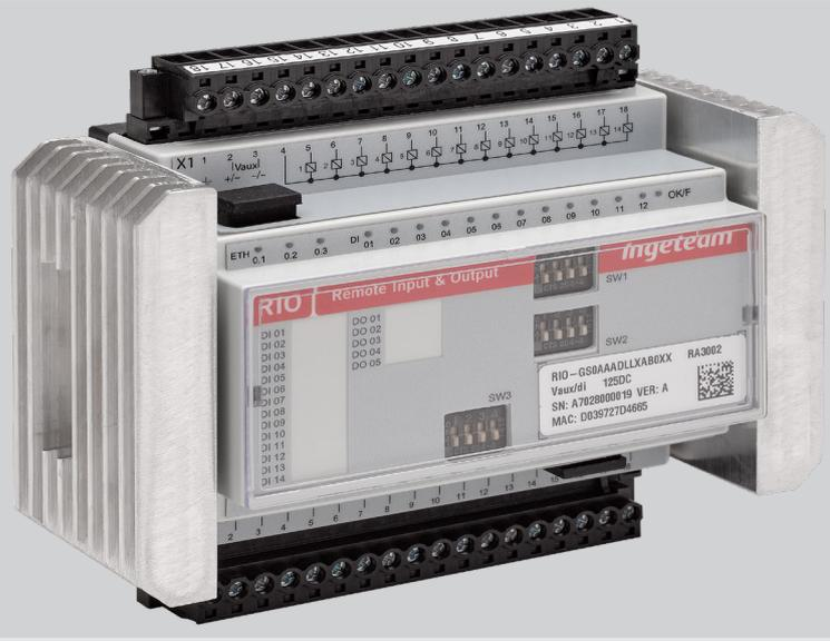
**INGEPAC™ RIO** is a digital input / output module which can be installed as a **control interface** to primary equipment in the switchyard and in MV switchgear cubicles. INGEpac™ RIO allows to the circuit breakers, disconnectors, transformers, etc. to interact remotely with the digital devices at substation automation systems.
