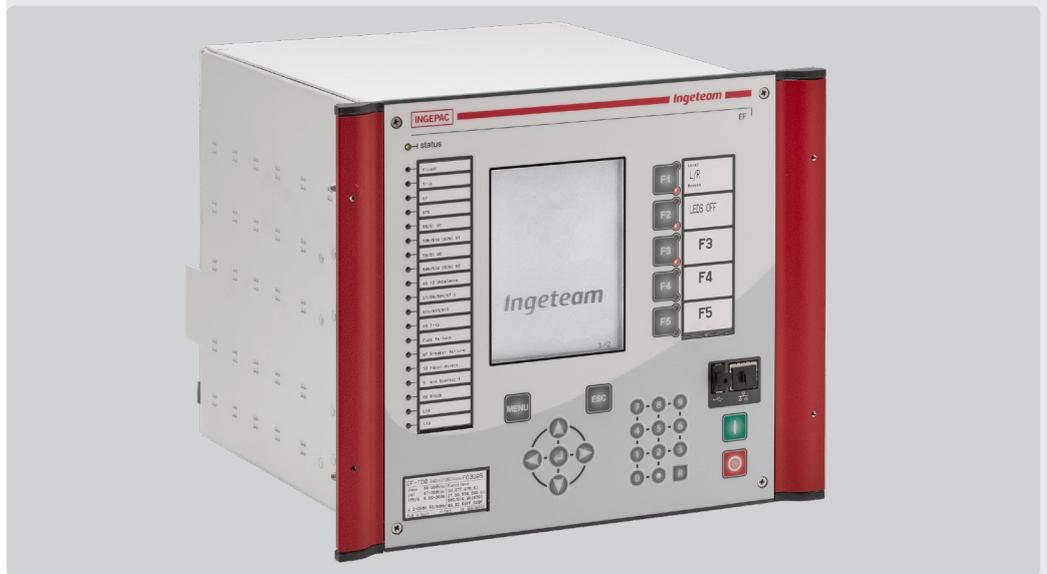
**INGEPAC™ EF TD** is a range of Intelligent Electronic Devices that provide all the **protection and control functionalities** required for two and three winding power transformers. It also provides **instantaneous and biased differential protection**, with harmonics blocking, as well as low impedance restricted earth fault.
