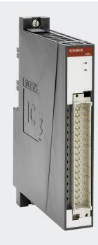
The IC3356 is an analog input measurement module, software configurable in voltage (-10V to +10V) or in current (-20mA to +20mA). All sixteen input channels have only a common reference point inside the module.
