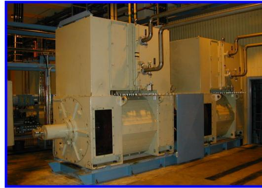
Tandem Arrangement Motors (Right Tension Reel)
