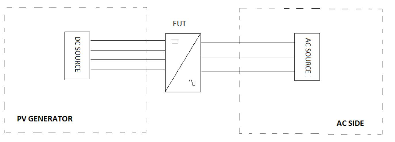
Different equipment has been used to take measures as it shows in chapter 2.3. Current and voltage clamps have been connected to the inverter output for all the tests.
