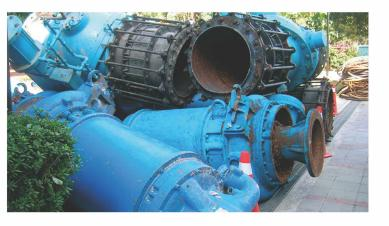
Again, Indar supplied environmentally friendly sets, lighter in weight, compact design ready to be installed (no alignment required), less wear and easier maintenance, less space required, less costly installation (geometry and reduced diameters), IP68 (no risk of electrical short circuit), self-lubricated and cooled, etc.
