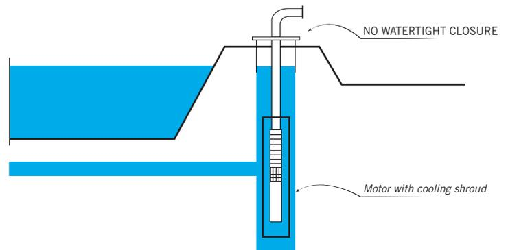
Figure 4. Reservoir Lifting. NO watertight with cooling shroud.
