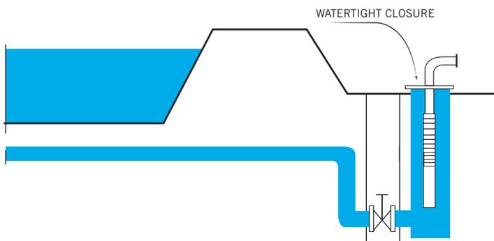
Figure 3. Reservoir Lifting. Watertight without cooling shroud.
