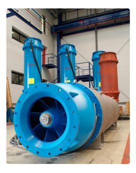
In this installation, the sets had to fulfil very strict operating requirements and their design had to be suitable for the existing electrical installation. Three duty points with a minimum hydraulic efficiency had to be guaranteed and other technical requirements were mandatory.
