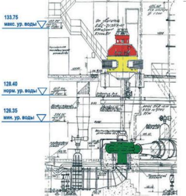
First lift pumping station of Zapadnaya water supply plant BEFORE modernization. Motors of pumps 36B-12M located below maximum possible water level of water reservoir.
