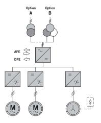
Redundant single-drive solutions: Applications which consists of motors doubly fed by two converters whose rectifier phase can be DFE or AFE.
