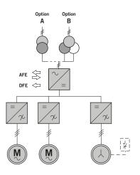
Redundant single-drive solutions: applications consisting of motors doubly-fed by two converters whose rectifier stage can be DFE or AFE.
