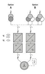
Single-Drive Solutions: Standard applications based on a single motor fed by an AFE or DFE converter.
