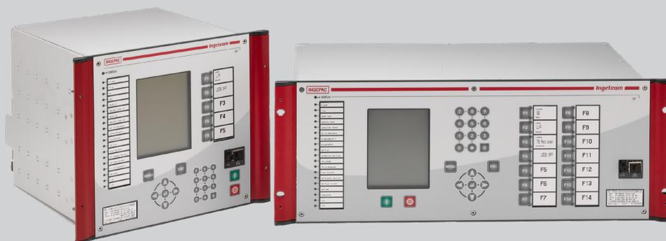
INGEPAC™ EF ZT is a distance protection relay with five independent zones of operation on which **MHO** or **quadrilateral** characteristic can be set independently, suitable for transmission lines, or **multibreaker configurations** such as, breaker and a half or ring. It determines the **type of fault**, differentiating among three-phase, two-phase and earth faults.
