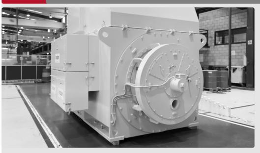
Indar is characterised by its capacity to manufacture large drives for different markets and applications. The INDAR SM family of synchronous motors is a clear example of this capacity. All of the motors in the SM series can be fed both directly from the electrical grid and from frequency converters.
