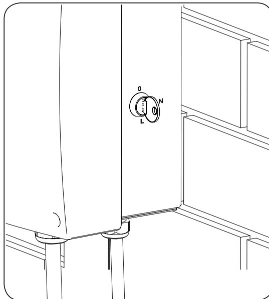
However, if deferred charge is activated using a USB memory, it becomes operative. In this case the *limited charge* deactivates, replaced by the deferred charge. Therefore, to select the deferred charge on the station, select position *L* using the key. Position *N* can still be used to select *nominal charge*.
