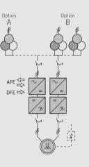
Multi-drive solution: Multidrive application in which several inverters are connected to one single DC bus. While some motors can be braking, others can be motoring, thus transferring energy between themselves through the DC bus (i.e. tension reels on reversing cold mills in the metal industry and test bench applications).
