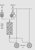
Redundant single-drive solution: an application consisting of a motor with two windings fed by two inverters. The rectifier side can be DFE or AFE.
