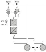
Redundant single-drive solution: an application consisting of a motor with two windings fed by two inverters. The rectifier side can be DFE or AFE.
