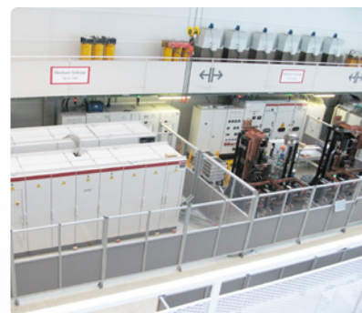
SSSC testing at Ingeteam's high voltage laboratory
