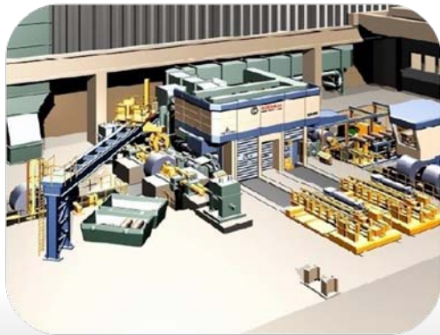
Double rolling mill ARCELORMITTAL
