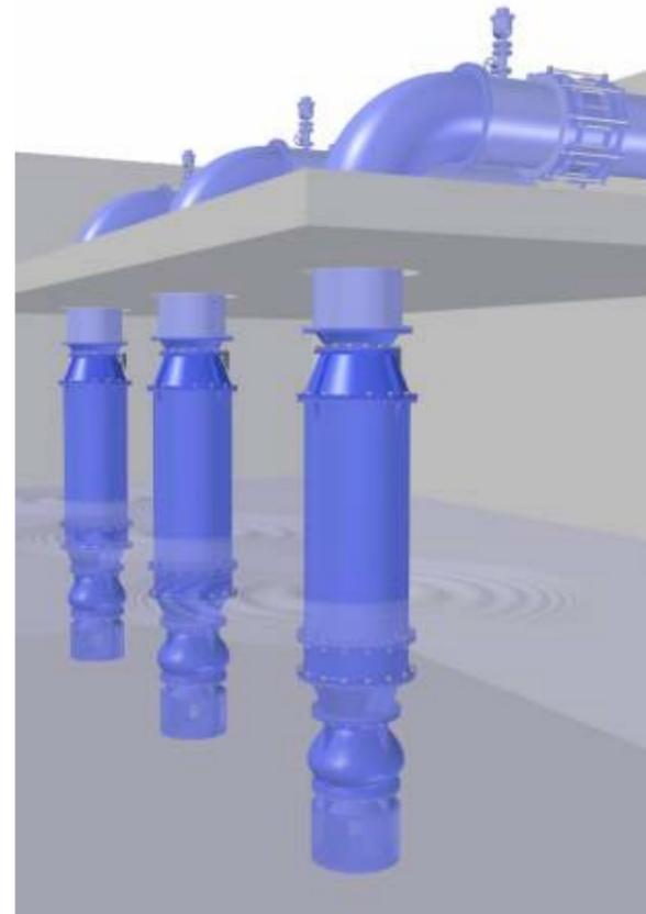
For such cases of application, INDAR has developed submersible pump sets with the relative position of motor and pump inverted.
