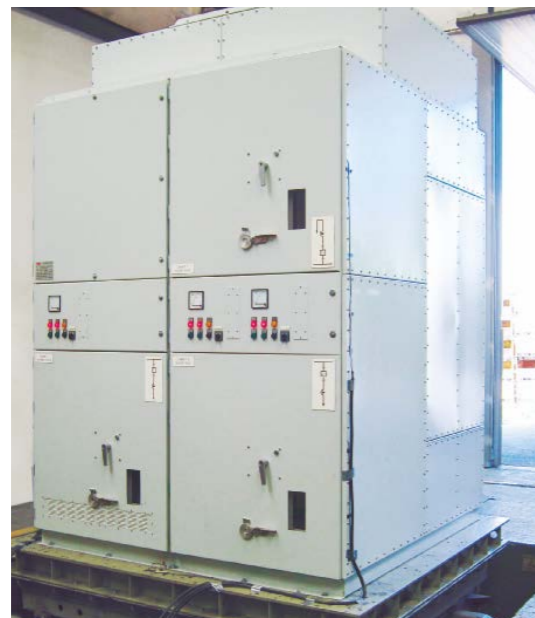
During Pine MV switchgear seismic test
