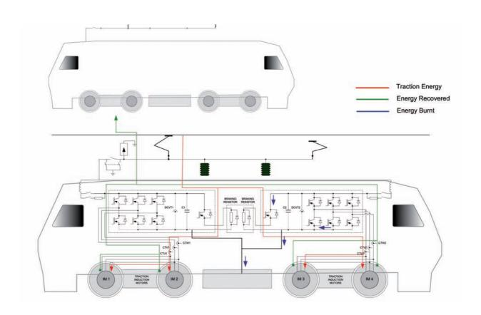
It is now normal for the rolling stock to incorporate regenerative braking systems which enable the energy generated during braking to be returned to the catenary.
