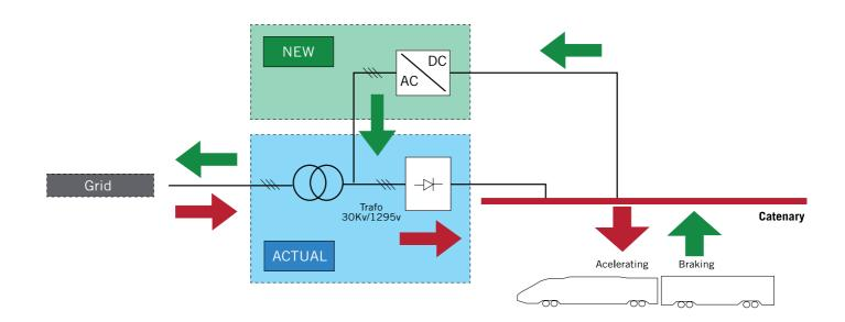
The INGEBER system developed by Ingeteam enables all the limitations associated with the return of energy from the units to be overcome.
